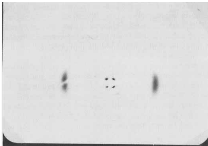
FIGURE 1 X-ray-pattern of 2 at room temperature (oriented sample).
